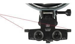
7. Using the condenser lens and vertical aiming beam knob located beneath the dust cover assembly, focus and position the aiming beam in the center of the illumination field already projected on the patient's forehead.
