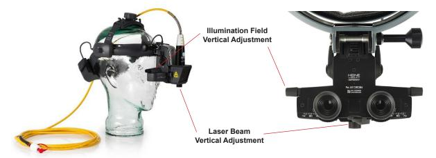
Figure 2. Adjustment Controls
