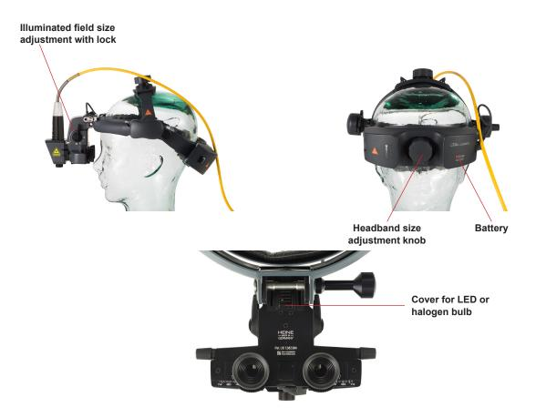
One pair of zero-diopter lenses is included with the TruFocus LIO Premiere. If desired, you may replace these lenses with the two-diopter lenses that are factory-mounted in the binocular eye pieces.
